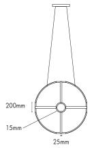
Suspension light Туре Material Solid brass Environment Indoors Ø 1070 mm Dimensions 2000 mm Cable Length Weight 9 kg Certification IP20 CE
