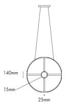
Suspension light Туре Material Solid brass Environment Indoors Ø 754 mm Dimensions 2000 mm Cable Length 7 kg Weight Certification IP20 CE Lamping
