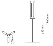
Floor light Туре Material Brass Environment Indoors Dimension 1160 mm Cable Length 1500 mm Weight 1.6kg Certification IP20 CE EU/UK 230 V Ceiling Rose 3 x linear opal LED \$14s\*, 3 x 9 W, 2700 K,
