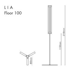
Floor light Туре Material Brass Indoors Environment 2150 mm Dimension 1500 mm Cable Length 2.3 kg Weight Certification IP20 CE 230 V EU/UK 3 x linear opal LED S14s\*, 3 x 16.5 W, 2700 Ceiling Rose
