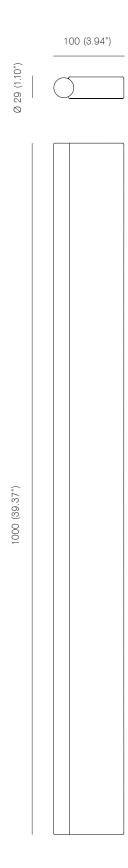
Bulb specifications 240V S14s opal LED tube Radium Raledina 16,5W / 1000mm ø29mm 1000lm / 2700K
