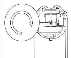
When tuning power back on, you can dim the light directly on the fixture with the knob under the disk. (120V instalation ONLY)
