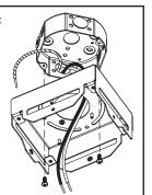
4 Make appropriate connextions with wire bundle provided to ceiling wiring. (Shut off main power at the circuit breaker panel)
