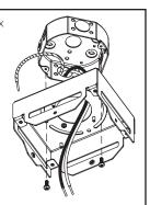
4 Make appropriate connextions with wire bundle provided to ceiling wiring. (Shut off main power at the circuit breaker panel)
