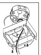
3 Make appropriate connextions with wire bundle provided to ceiling wiring. (Shut off main power at the circuit breaker panel)
