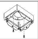
6 Pass the flat cable in strain relief in canopy and screw it in place. (Loosen captive screws for better passing of cable)
