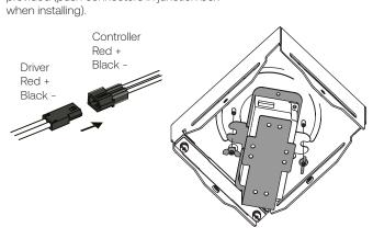
5 Screw support backplate on ceiling. (Screws not included)
