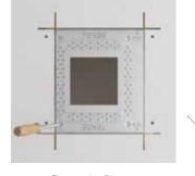
Cut a 225 x 192 x 65 mm rectangular hole in the wall and install 2 wooden planks
