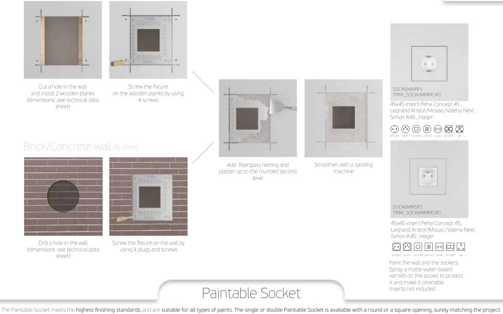
The Trimless wall box needs to be ordered separately. The wall box is both **easy to install** (glued or screwed via pre-drilled screw holes/large mounting surface to easily adjust) as well as **easy to plaster** thanks to the rounded second level in the Xillo fixture. The wall box is available in 6mm and 12,5mm thickness.
