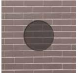
Drill a ø 145 mm hole in the wall
