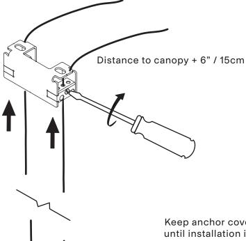
Keep anchor cover wrapped until installation is complete.
